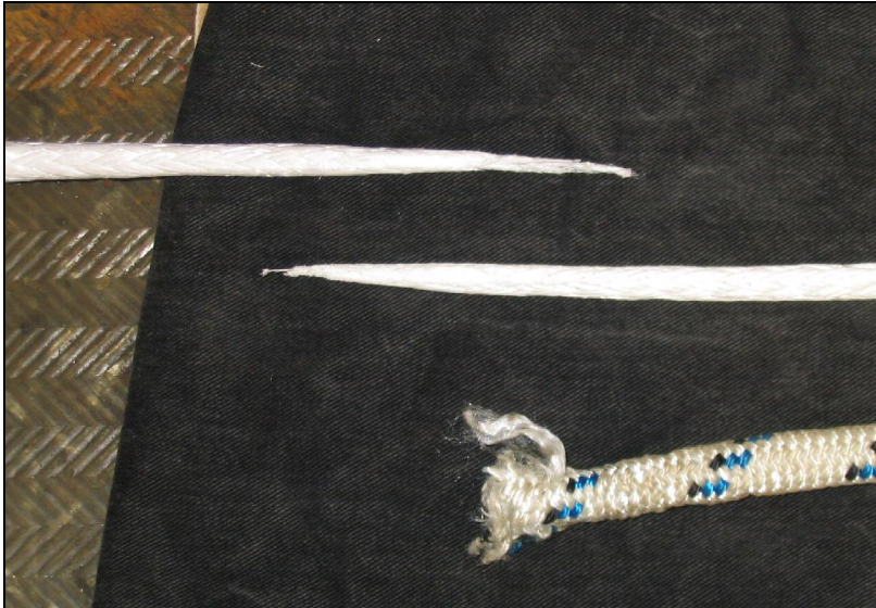
Figure 7. Failed Spectra rope.
