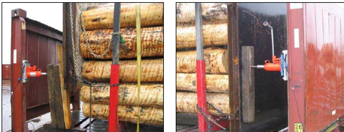
Figure 11. Friction test set-up.
