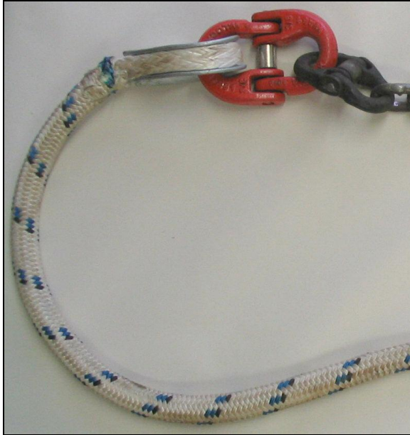
Figure 5. Spectra/Kevlar rope lashing.
