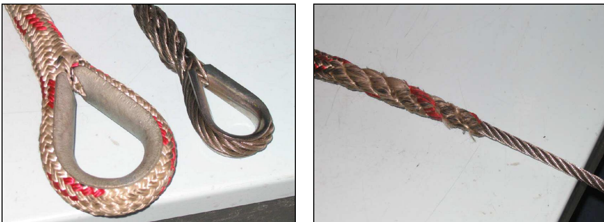
Figure 8. Alternative Spectra/Kevlar rope damage prevention.
