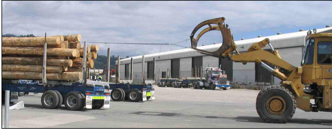
Figure 12. Log friction coefficient determination using the pull test.
