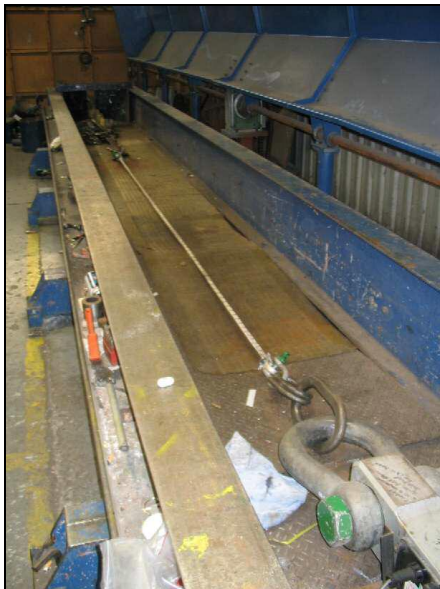
Figure 6. Spectra rope tensile test set-up.
