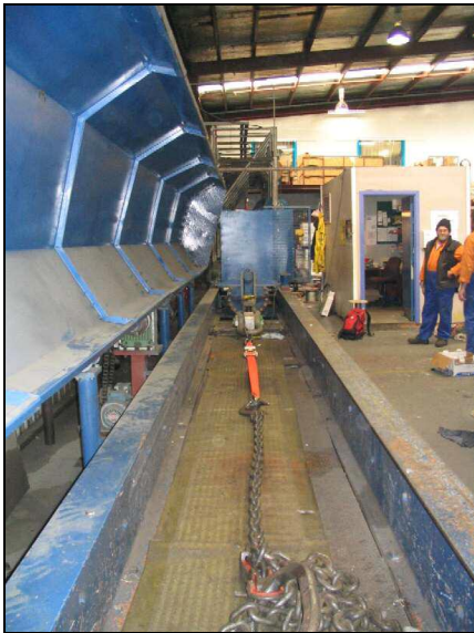
Figure 4. Flat bed test set-up for web tensioner tests.
