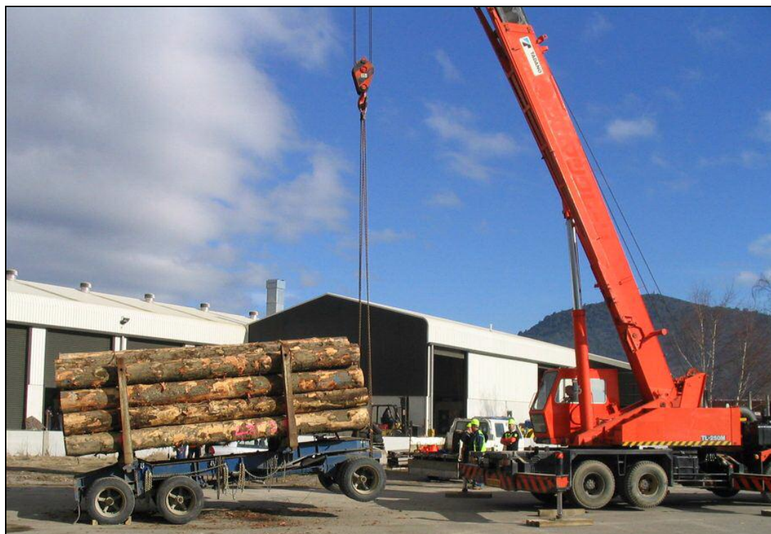
Figure 2. Tilt testing the load restraint system.
