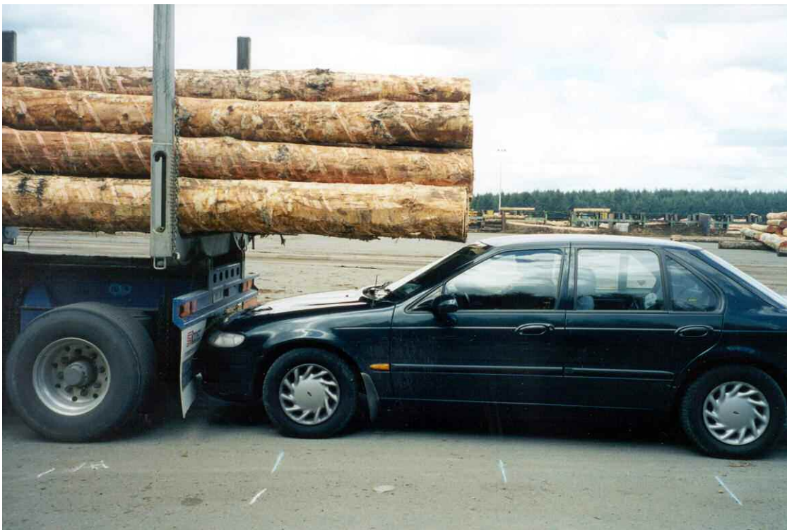
Photo 9 Underrun situation – Falcon
