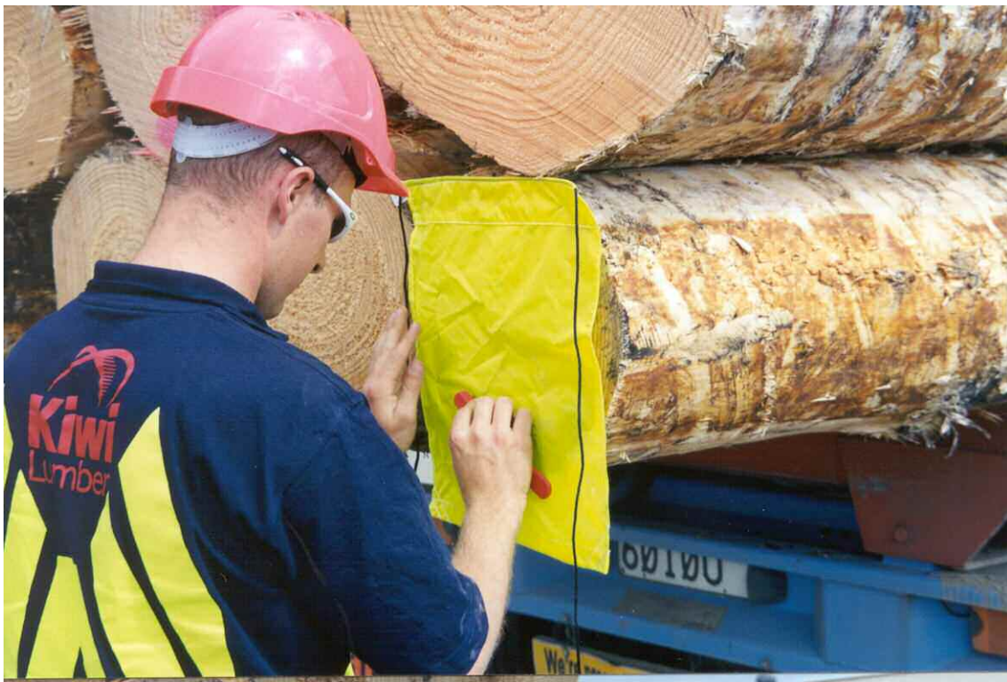
Photo 12 Reliance on office staples to secure the load
