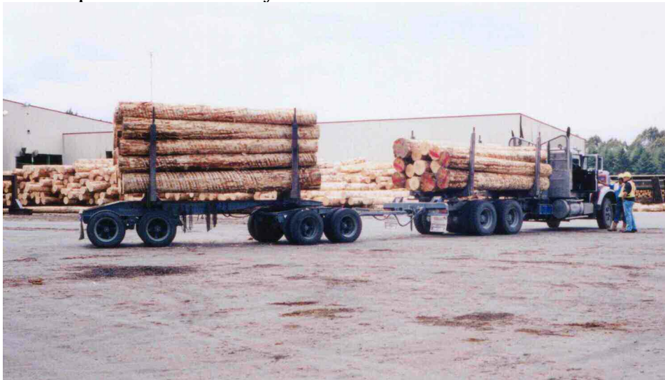
Figure 6. "Shorts" combination loaded with 4.95m saw logs.
