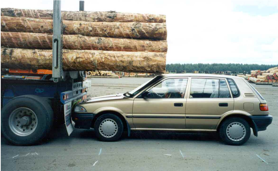
Photo 10 Underrun situation - Corolla
